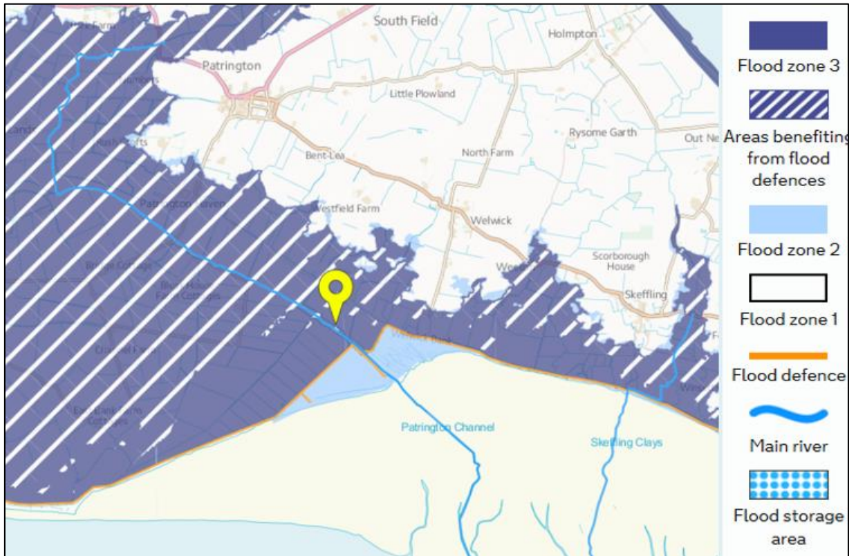
Plate 6.7: Current flood risk at Outstrays to Skeffling (source: Environment Agency, 2018 3 )
